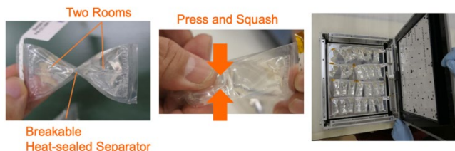
Fig.2 Experimental setups. A sample bag having a breakable separator, and sample box equipped with UV LEDs.
