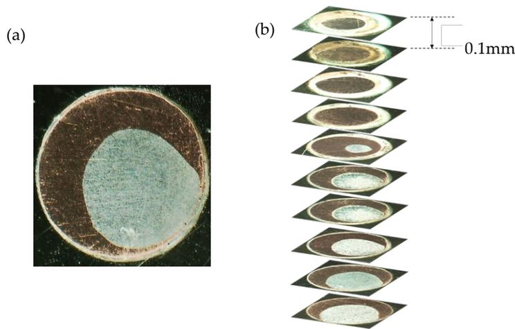
**Fig. 3** (a) Examples the cross section at Fe-50 mol%Cu and (b) the cross section at Fe-50 mol%Cu using the parallel projection method
