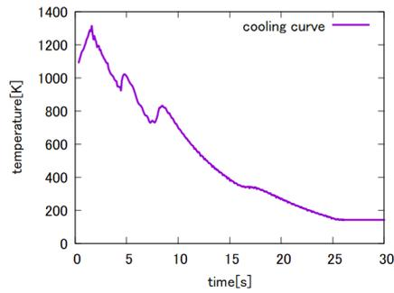
**Fig. 2** The cooling curve at Fe-50 mol%Cu
