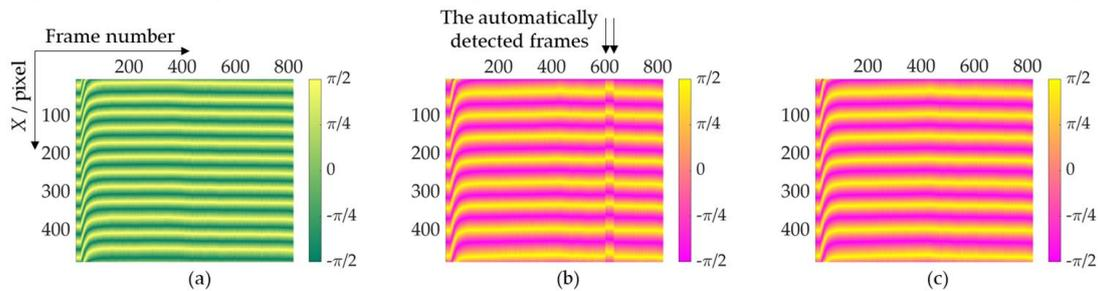
**Fig. 1** The phase spatio-temporal images in *Run #2-16* at (a)  $532$  nm, (b)  $780$  nm with hopping, and (c)  $780$  nm applied the hopping correction method: frames were taken every  $6$  s for the first about  $0.6$  h of the  $9$  h-experiment, and every  $66$  s thereafter.
