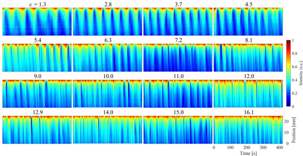
**Fig. 2** Spatiotemporal temperature map with over critical parameter  $\varepsilon$
