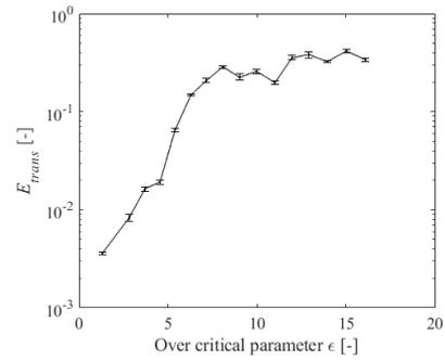
**Fig. 4** Variation of Translation error  $E_{trans}$  with over critical parameter  $\epsilon$
