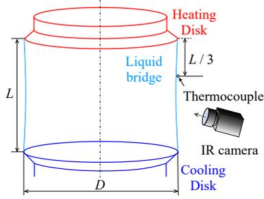
**Fig. 1** Schematic diagram of liquid bridge setup
