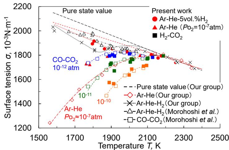
Figure 1 Temperature dependence of surface tension of molten iron
