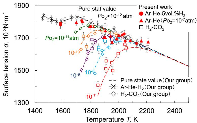
Figure 2 Temperature dependence of surface tension of molten nickel
