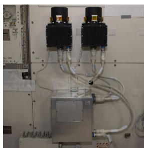
Fig. 1 Photo of the PS-TEPC in the ISS. The two black boxes of the upper side are Detector Units (DU) and the silver box of the lower side is the Control Unit (CU). Three dimensional tracks of incident particles in the DUs are reconstructed from the signals obtained in the data acquisition system in the CU.
