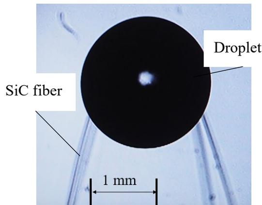
Fig. 4 Droplet supported by the SiC fiber
